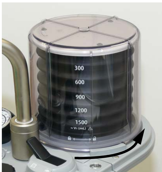
FIGURE 7-5 Removing the Bellows Dome
