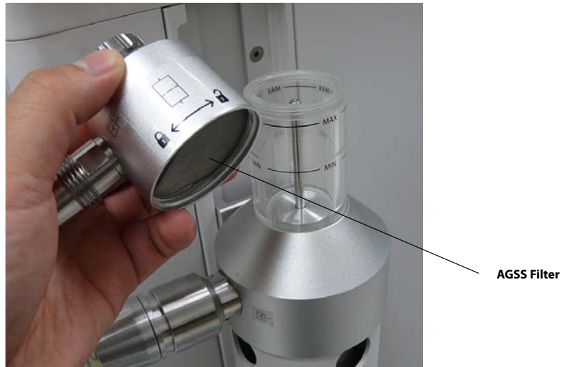
FIGURE 7-26 Removal of AGSS Top / AGSS Filter Inspection
