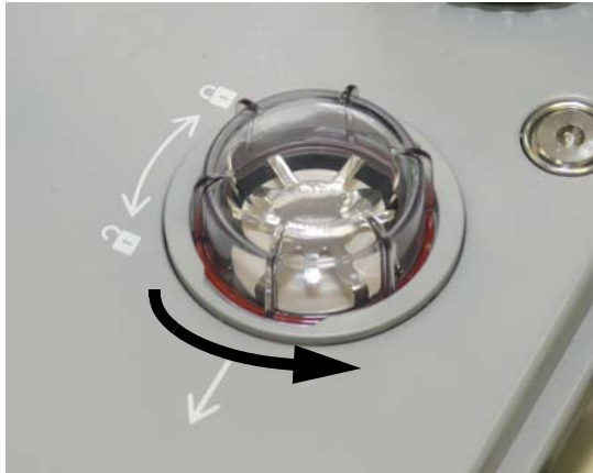
FIGURE 7-11 Valve Dome Removal
