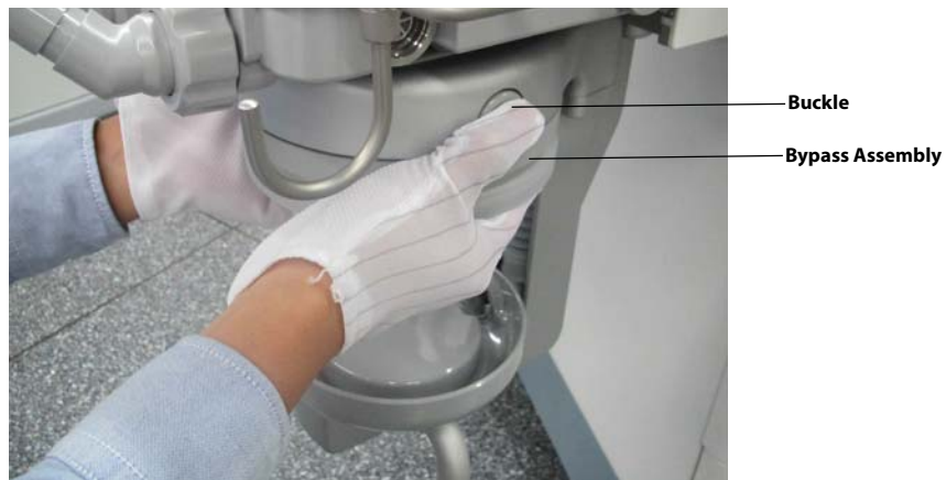
FIGURE 7-21 Remove Bypass Assembly
